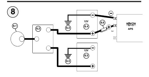
Advanced 12VDC Vehicular Battery Connection. See Pg.8. 8.1 is the alternator. 8.2 is a battery isolator. 8.3 is the vehicle battery ground. 8.4 is an auxiliary vehicle battery. 8.5 is the vehicle battery. 8.6 is the fuse.
